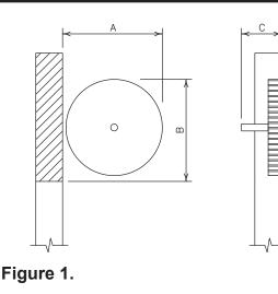
TEK SCREW THE NARROW JAMB PLATE IN USING THE DIMENSIONS SHOWN
