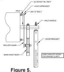
5.3 Slide the chain hoist assembly on the axle and align the sprockets parallel to each other.
